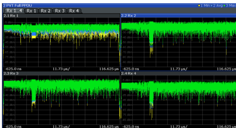
Fig. 3-19: PVT Full PPDU result display for IEEE 802.11n MIMO measurements
